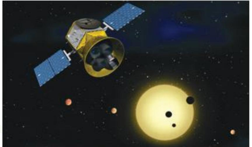
The TESS satellite uses an array of wide-field cameras to perform a survey of 85% of the sky.
